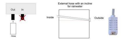
The cover of the outer hose should be mounted downward as shown in the picture on the right.
